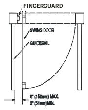
ELEVATION SHOWING ALLOWABLE DISTANCE FROM GUIDERAIL TO DOOR
